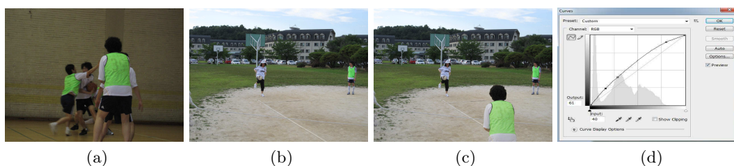
Figure 7: Cut-and-paste image forgery using Photoshop. (a) The original image from which an object is cut, (b) the original image onto which the cut object is pasted, (c) the composite image and (d) parameters of Photoshop Curve Tools.
